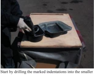
Start by drilling the marked indentations into the smaller extension, then align the extension to the AC Delete cover, and drill the remaining holes. (as shown above)
