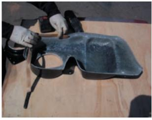
Next, use either the 3M silicon, or the windshield ribbon to provide a good seal from the extension to the AC Delete cover.
