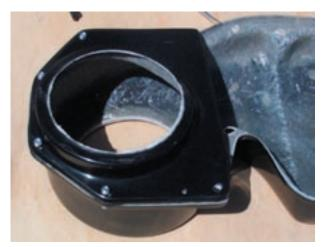
Attach the extension to the new AC Delete cover using the nuts provided. To keep the nuts from coming loose use a small amount of silicon on the end of the screw.
