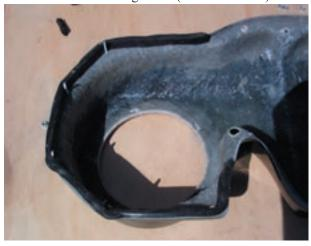
Using the hardware provided (#6 machine screws and nuts) insert the screws making sure not to brake the bead of silicon or ribbon.
